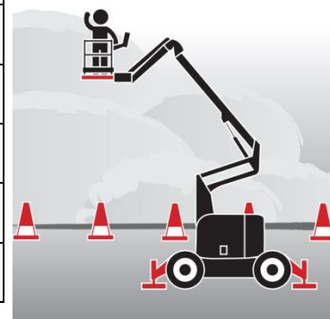
• Set outriggers, brakes and wheel chocks, even if on a level surface. • If working near traffic, set up work zone warnings using cones and signs. • Stand on the floor of the bucket. Do not climb on or lean over guardrails.
